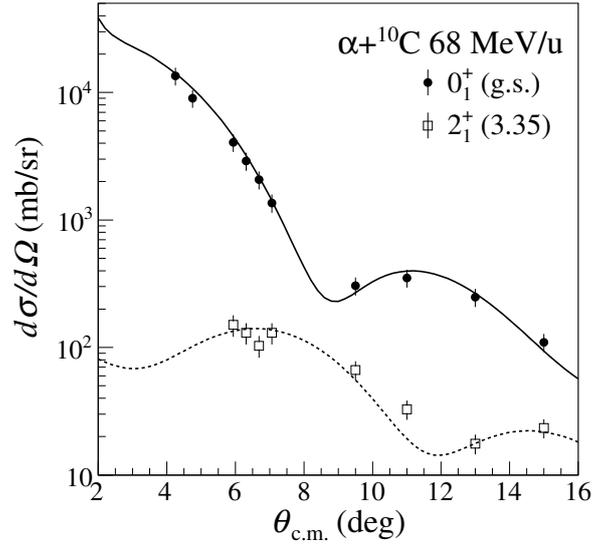
Figure 4: Differential cross sections of the  ${}^{10}\text{C}+\alpha$  elastic (solid circles) and inelastic scattering to the  $2_1^+$  state (open squares). The solid line and dashed line represent the optical model and DWBA calculations, respectively.
