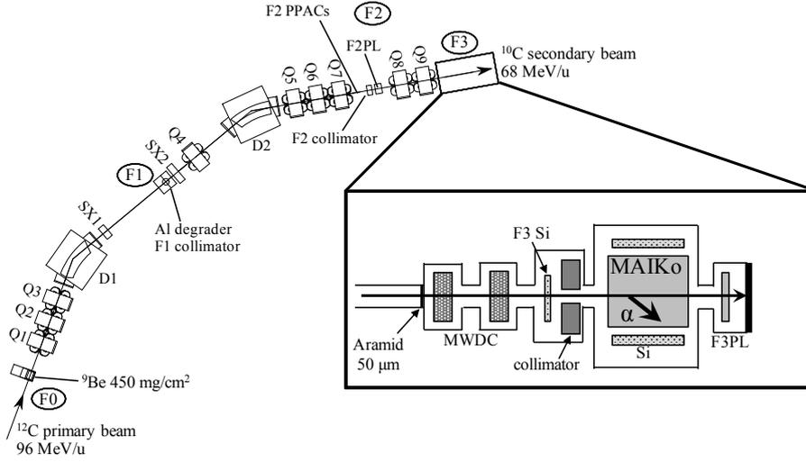
Figure 1: Experimental setup of the  $^{10}\text{C}(\alpha, \alpha')$  measurement at the EN beamline.
